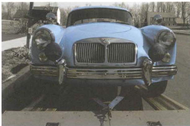
Loading a trailer alone is a lot easier when using a bridle harness and a winch. The combination allows you to inch the car up the ramps while ensuring it's properly aligned. Photo by Jay Tester
